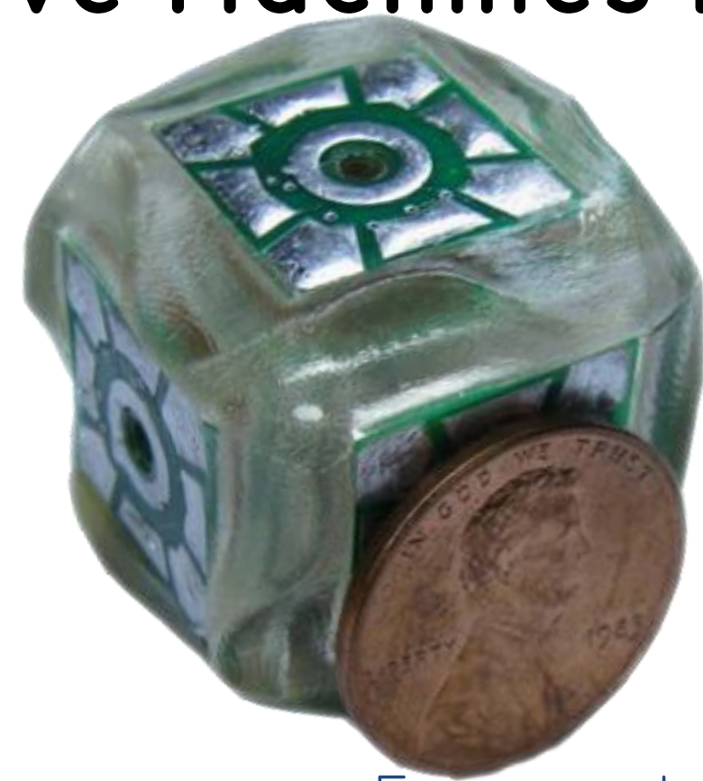
Each module consists of an 3D-printed skeleton, 12 conventional circuit boards, one flexible circuit board and 6 fluidic valves.
